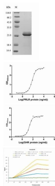
(Tris-Glycine gel) Discontinuous SDS-PAGE (reduced) with 5% enrichment gel and 15% separation gel.
